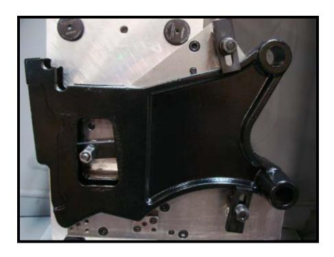
The austempered ductile iron casting is machined at Dotson's in house machining facility after austempering (300 hardness brinnell) on a Makino horizontal CNC machining center. The ADI part is twice as strong as the steel weldments it replaced.
