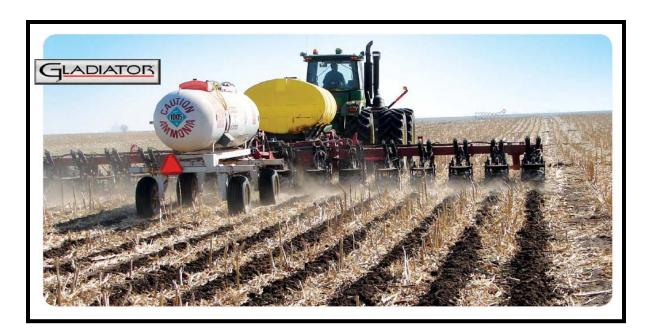
The perpendicular alignment of the shank pivot mount to the implement tool bar is important as twist in the shank can cause an uneven pull causing the implement to track off course. This can cause inefficiencies in a strip till application. Accurate row spacing places the nutrients only where the plant needs it, resulting in yield improvements up to 50%. The alignment is important for even wear on the shank along with the point and allows minimal soil fracture to more easily seal fertilizer.
