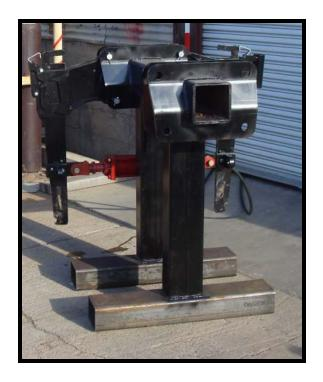
The parts, both welded and ADI casting, were anchored to a bar where a 4,000 PSI hydraulic cylinder was mounted between them and cycled till one of them broke or showed signs of wear or fatigue. While neither part actually broke the weldment showed signs of wear and fatigue around welds and other stress points, the casting looked like it just came out of the box. This was done with parts facing each other and parallel to one another, for side load testing.
