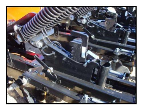
This Shank Pivot mounts to the implement tool bar and carries the main load of the Kuhn Krause Gladiator Precision Tillage System for Strip-Till application. The shank pivot mount casting carries the driving force as the shank is pulled through the ground. This force causes high stress on a welded steel fabrication where an ADI(Austempered Ductile Iron) casting prevails.
