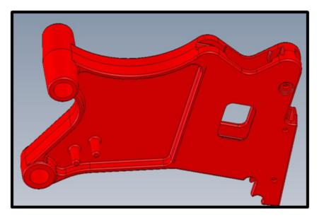
A single piece casting design was developed that included all the functionality of the previous weldment. This single center rib design or "I" beam style part reduced the number of cores required to produce the casting. This machined Austempered Ductile Iron part went from a 50.62 pound weldment to a 41.79 pound casting and was a 26% cost savings to the customer. The part is cast, austempered(Grade 1), painted and then machined to give the customer a stronger, lighter, more sleek, looking part.
