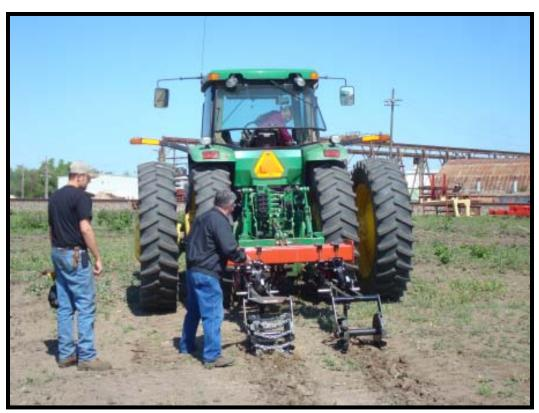
The parts were then mounted to another tool bar with a 300+HP tractor, set in the ground and driven into buried cement blocks to simulate impact. When the tractor came to rest the casting had once again prevailed and the customer was satisfied.
