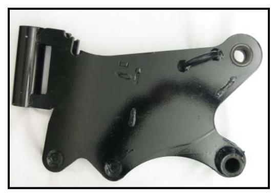
This ADI casting is a conversion from a fifteen piece weldment. Design enhancements were selected to produce the best casting design. Material was moved from outer portion of the part where welding has easier access to the centerline which in the casting process is more conducive to making a solid casting and eliminated necessary cores. The profile ribs serve a dual purpose of strength and also feeder paths to the three bosses.
