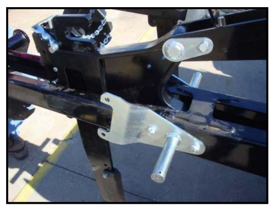
In converting the shank pivot mount to a casting, Krause alleviated burden on the weld shop and reduced back log of laser cutting machines.
