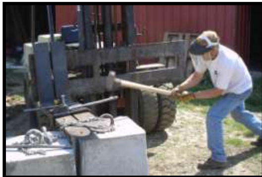
Mike Bergman testing the ductile casting
