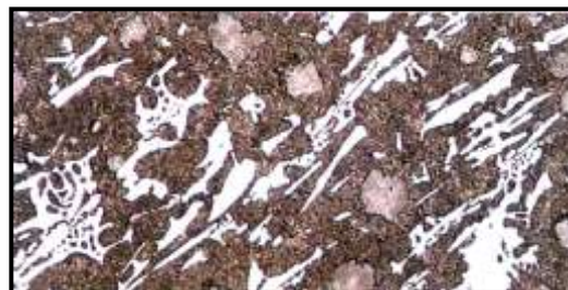
CADI matrix is ausferrite and carbides
