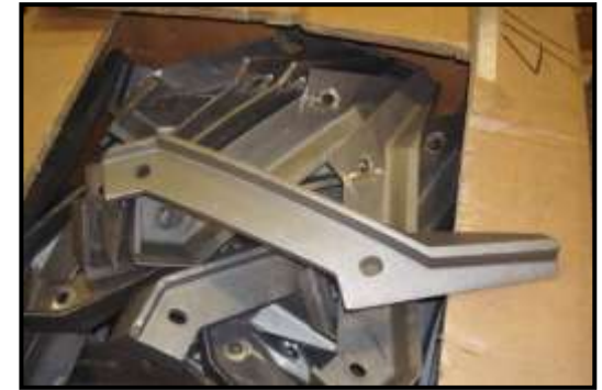
CADI parts going to Applied Process for heat treating
