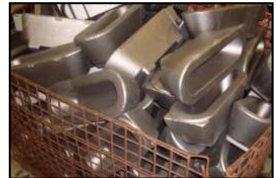
These are ingot molds for aluminum and copper industries
